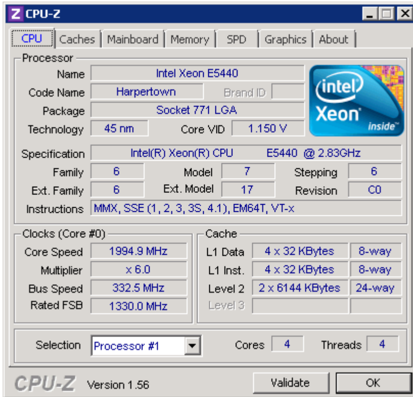
Figure 1.5: Intel Xeon E5440 information displayed in CPU-Z.
