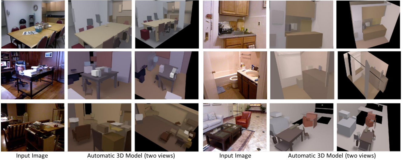
Figure 6: Examples of 3D models estimated automatically from the input RGBD images. The method is accurate for layout surfaces and large pieces of furniture. Small and heavily occluded objects remain a major challenge. Directions for improvement include incorporating object categorization and physical support estimation.
