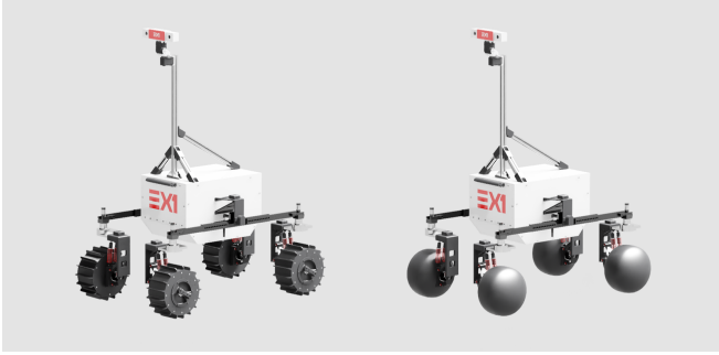
Fig. 5. Rover illustrated with visual wheel geometry (left) and physics wheel geometry (right).
