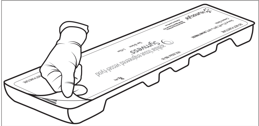
Figure 3a: Non-sterile operator pulls back the Tyvek® lid by the corner tab
