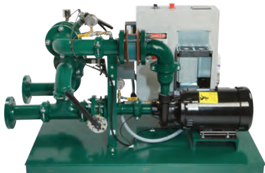
Variable frequency drive has improved operation for irrigation pumps across the industry, providing a constant pressure over a wide range of flows without the need for pressure regulation devices, says Kamas. Photo: Rain Bird
