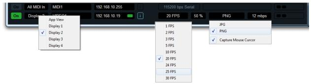
It can capture en entire display (from 4 connected screen – 4K resolution max) or the main window interface only (app view). It is done by sending PNG or JPG frame up to 30 times per second to the destination address through VBAN-Frame protocol.
