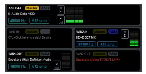
Sample Rate or buffer size displayed in dark blue means it is different from the master one. This should work anyway since the matrix audio engine is able to manage any kind of stream configured in different sample rate or buffering.
