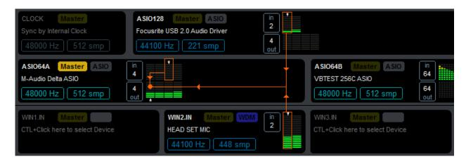
Click on OUT peak meter to see all inputs routed to this output. Click on IN peak meter to see all outputs getting audio from this input.
