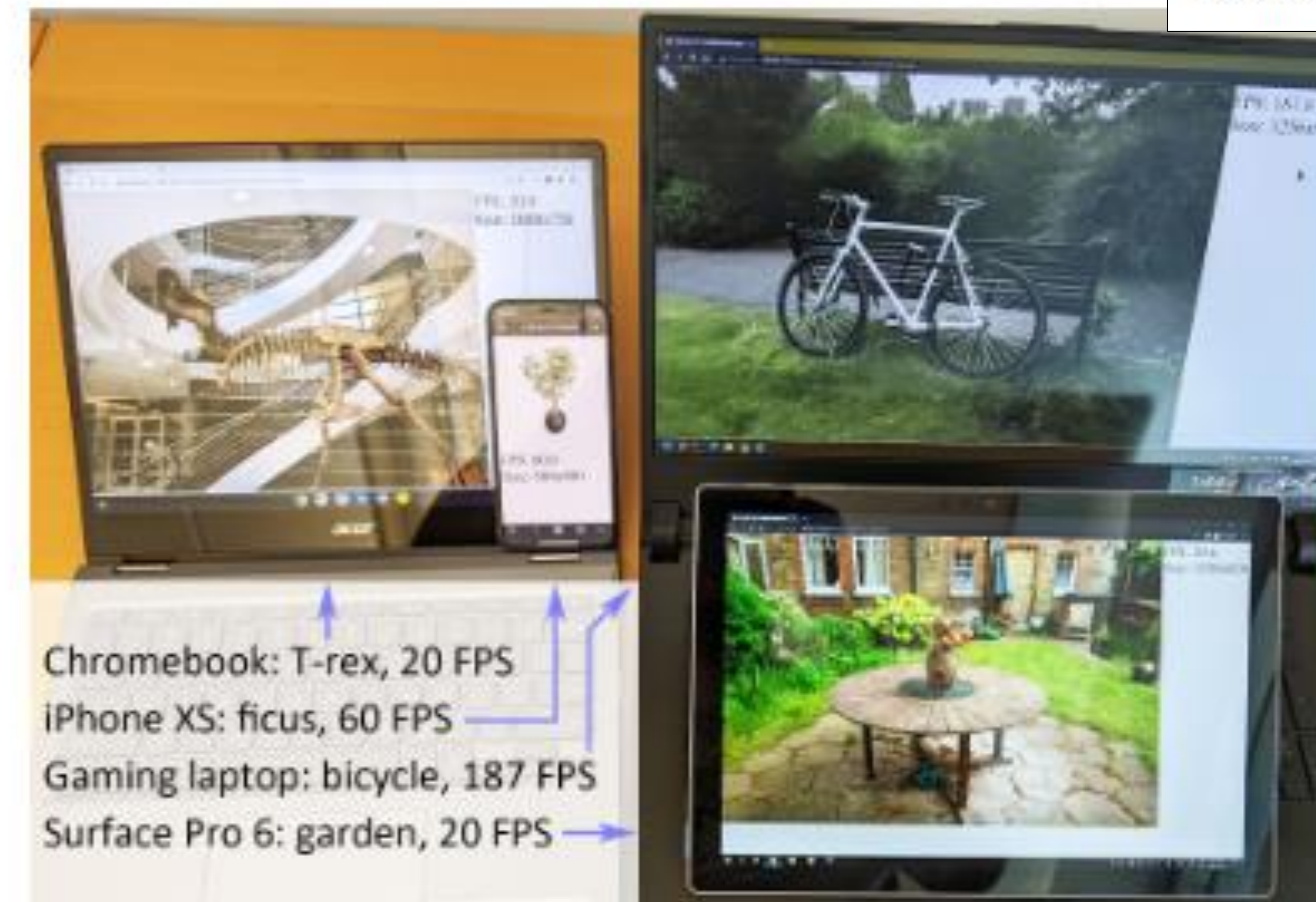
Figure 1. Teaser – We present a NeRF that can run on a variety of common devices at interactive frame rates.
