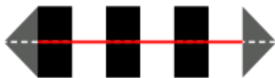
Figure 18-11. Stroke start or end point within a dash for flat dash caps
